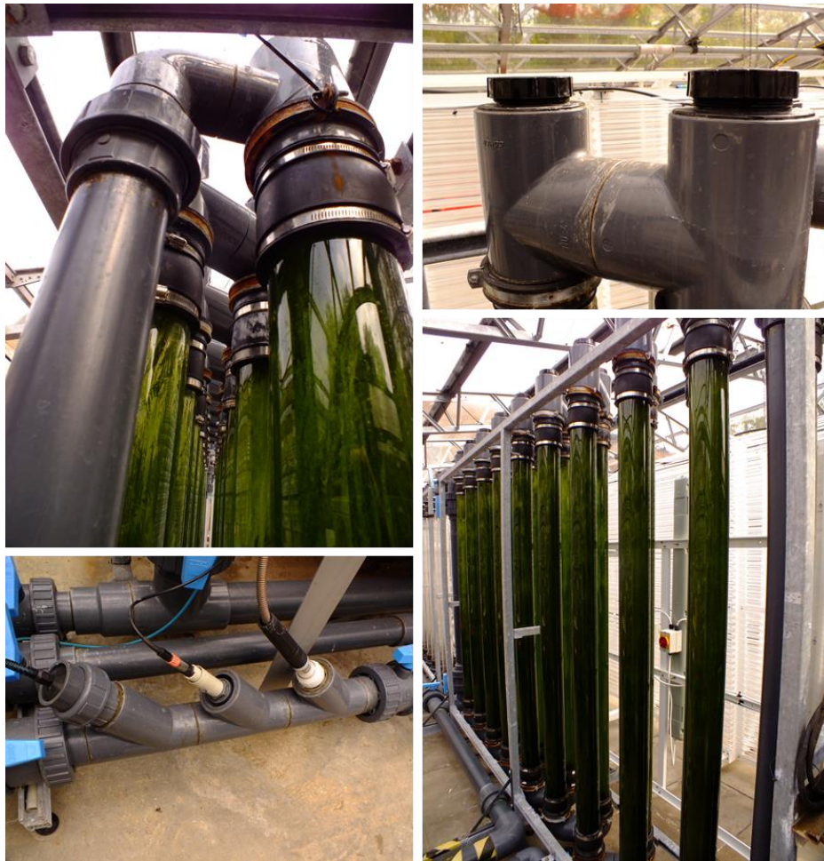
Fig.4.5. Custom made multiple vertical-tube reactor with a total volume of 1000L. The tube diameter is 12cm. These acrylic tubes are connected at top and bottom, so the culture is pumped through the whole system. Top-right shows the top caps, with degassing vents. Bottom-left shows the pH and \text{O}_2 sensors in the return-from-pump branch of the system. Although of potentially infinite expansion, this reactor design is not amenable to easy-cleaning, requiring the removal of the upper unions and the use of a brush (see upper panels of Fig.4.1).
